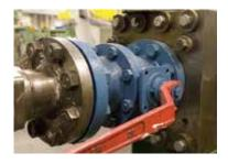
**Problem:** A mineral oil-based grease, exposed to harsh pipeline materials, hardened and caused difficult valve operation as well as material leakage past the valve seat and seals.
